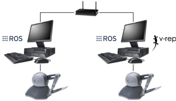
Fig. 3- Experimental setup for cooperative haptics teleoperation.
