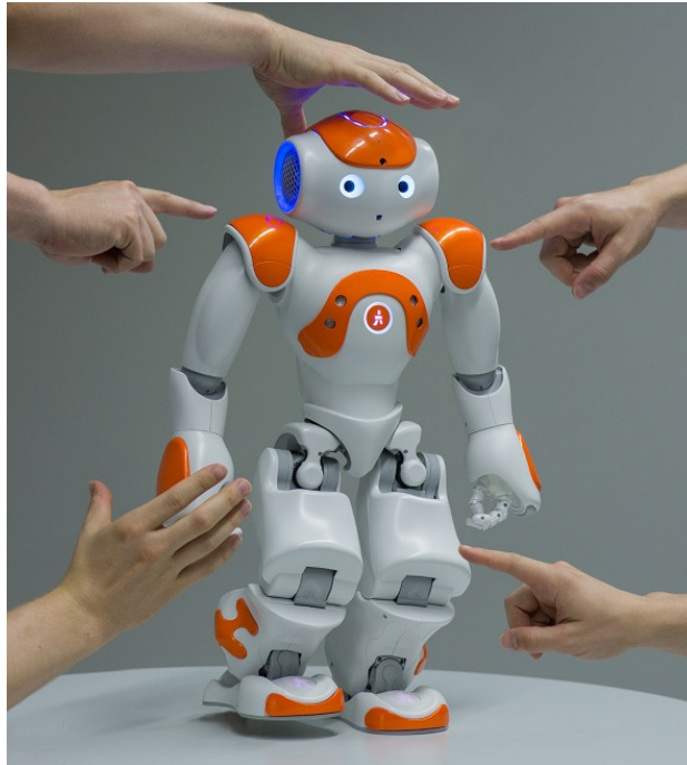
Fig. 1: A NAO robot estimates the influence of external perturbations applied by a human interaction partner to its current behavior execution.
