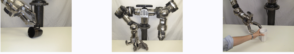
Fig. 1. Potential Manipulations faults. (left) Missed grasp. (middle) Heavy object. (right) Uncontrollable obstacle.
