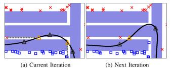
Fig. 3: Part of the learned manifold and points sampled on the manifold, before and after we add the two  $C_{\rm free}$  manifold points (yellow triangles) to the planning graph. The  $C_{\rm free}$  manifold points connect to their nearest neighbors in the planning graph (shown with dashed lines), and become part of the training data in the next iteration.
