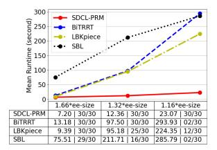
Fig. 5: Compare 7-DOF scenes with different hardness levels. Table is showing "average runtime (s)  $\mid$  solved cases". 30 trials for each planner and each difficulty level.
