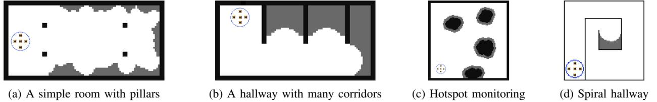
Fig. 3: Maps of the simulated environments used in our experiments. All robots start within the blue circle with the base station in the center of the circle. Gray points are unknown space.
