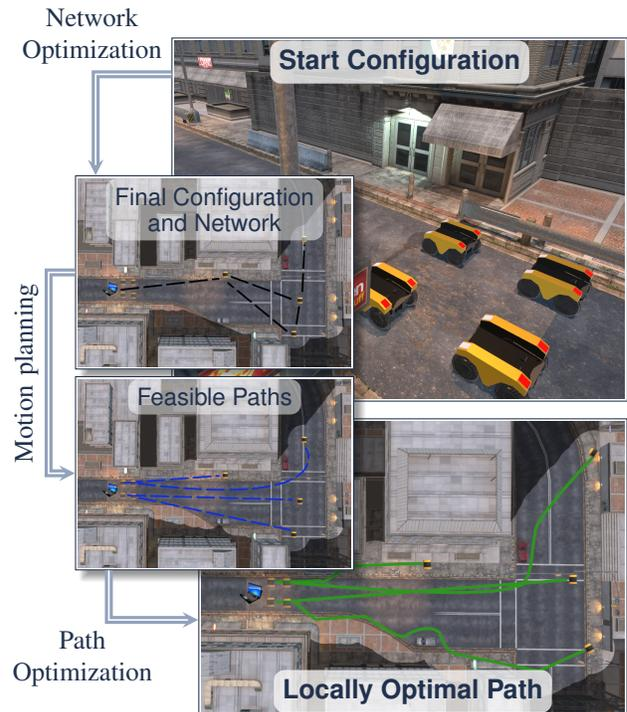
Fig. 1: A robot team exploring an urban area. Unknown regions are shown in black. Our algorithm optimizes information gain while maintaining communication between the team and base station.
