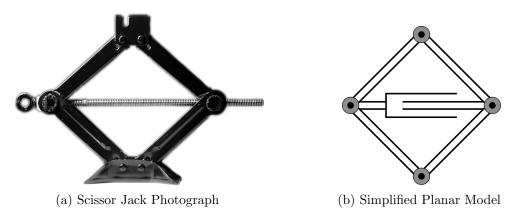
Figure 1: Scissor Jack Mechanism
